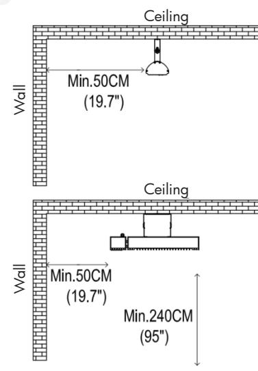
The heater must be installed at least 1.8 meter above the floor.
