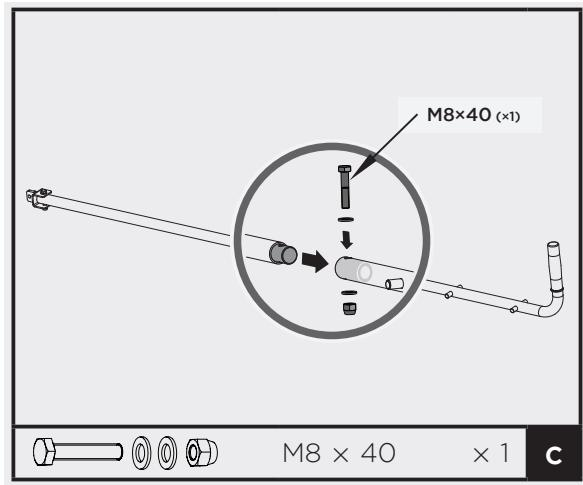
4. Attach control lever to the guide tube. Line up holes and fasten with M8×35 bolt, washers and nut.
