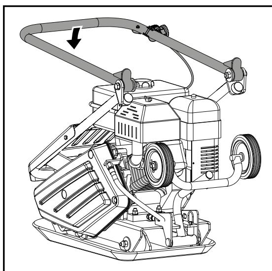
7. Carefully fold the upper handle down. Do not allow control cables to become pinched or bent.
