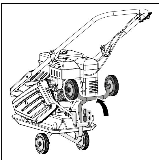
6. Pull up the spring bolt and fold up the wheels bracket.
