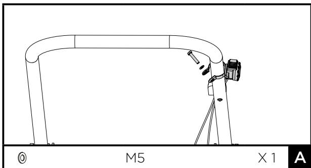
Unscrew bolt 5x35 from throttle control. Secure the throttle control onto the upper handle with a flat washer 5 and the bolt 5x35 that just were unscrewed.
