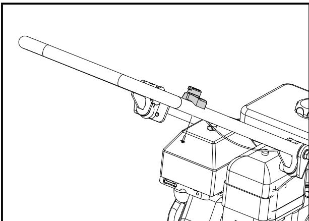
Remove the screw from stop switch, align the hole in handle with hole in switch. Insert the screw into the hole and tighten in the switch.
