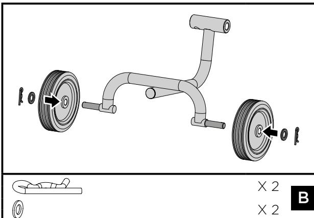
1. Slide the wheels over the stub axles. Secure with hairpin retainers and flat washers.
