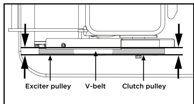
4. Push engine toward the back of the plate by turning the adjustment bolts A to remove any slack in V-belt.
