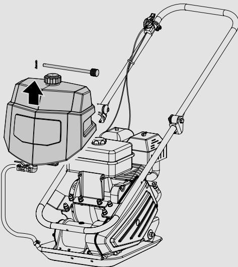
1. Remove the metal cover or water tank.
