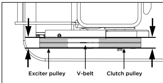
3. Slide the engine toward the front of plate and slip the old V-belt off of the wheel pulley and install the new V-belt in its place.
