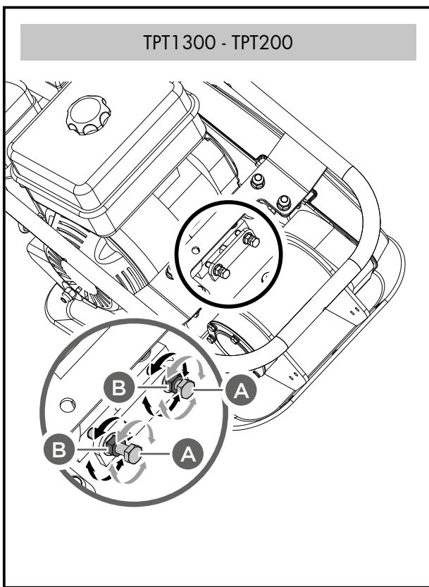
3. Loosen the jam nuts B, leaving enough space between the nut and bracket.
