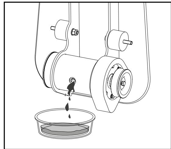
5. Remove pipe plug from top of exciter housing. Tilt housing upside down so oil drains from exciter. Examine oil for metal chips as a precaution to future problems.
