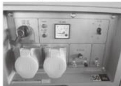
Before starting the generator, make sure the air switch is in the OFF position.
